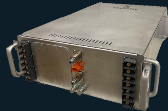
80 kW energy router module (36" x 10" x 24")
