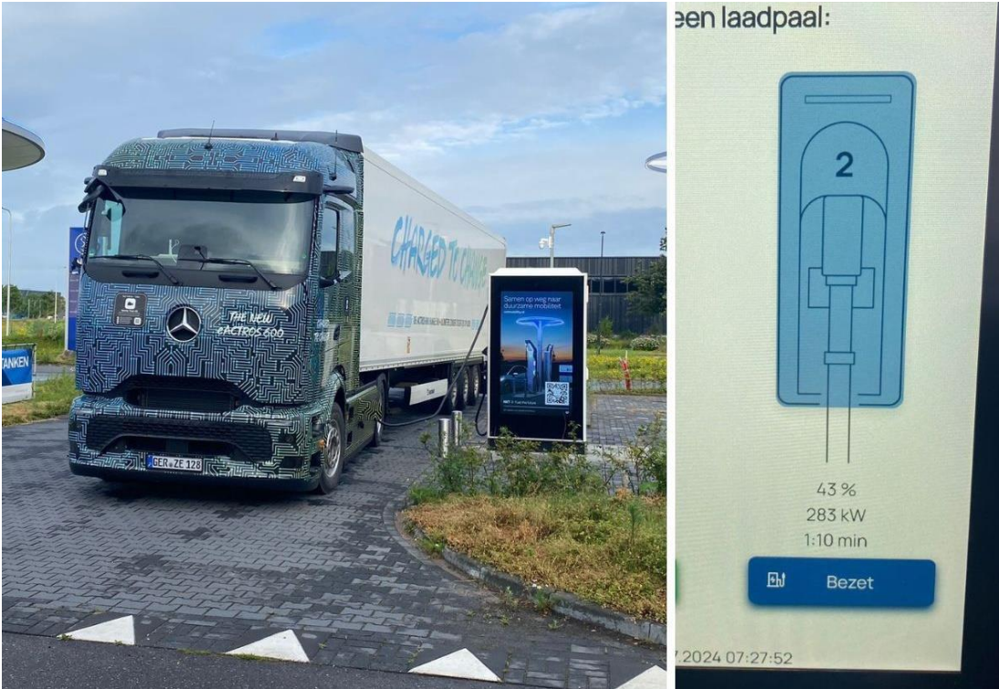
283kW charging power with only 40kW input power (at ChargePost)
